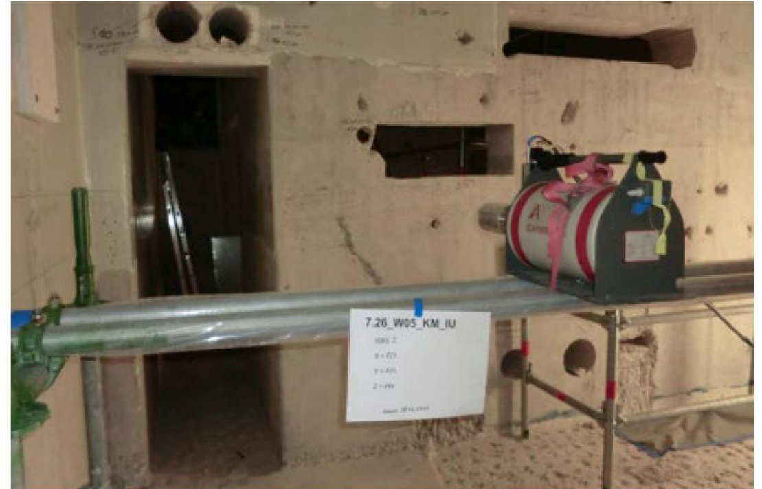
Figure 10: In-situ gamma spectrometer for decision measurements of buildings (Brenk Systemplanung GmbH)
